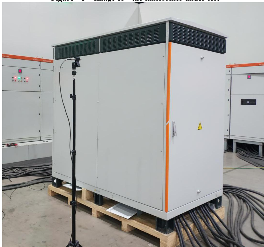
Figure 4 Image of the inverter under test
