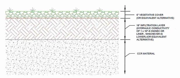
§257.102(b)(1)(iii): If closure of the unit will be accomplished by leaving CCR in place, a description of the final cover system, designed in accordance with paragraph (d) of this section, and **the methods and procedures to be used to install the final cover**. The closure plan must also discuss how the final cover system will achieve the performance standards specified in paragraph (d) of this section.
