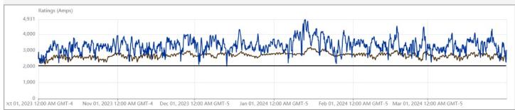
Chart 2. Time Series of Line 345kV-1 line ratings, including DLR, AAR, and static ratings
