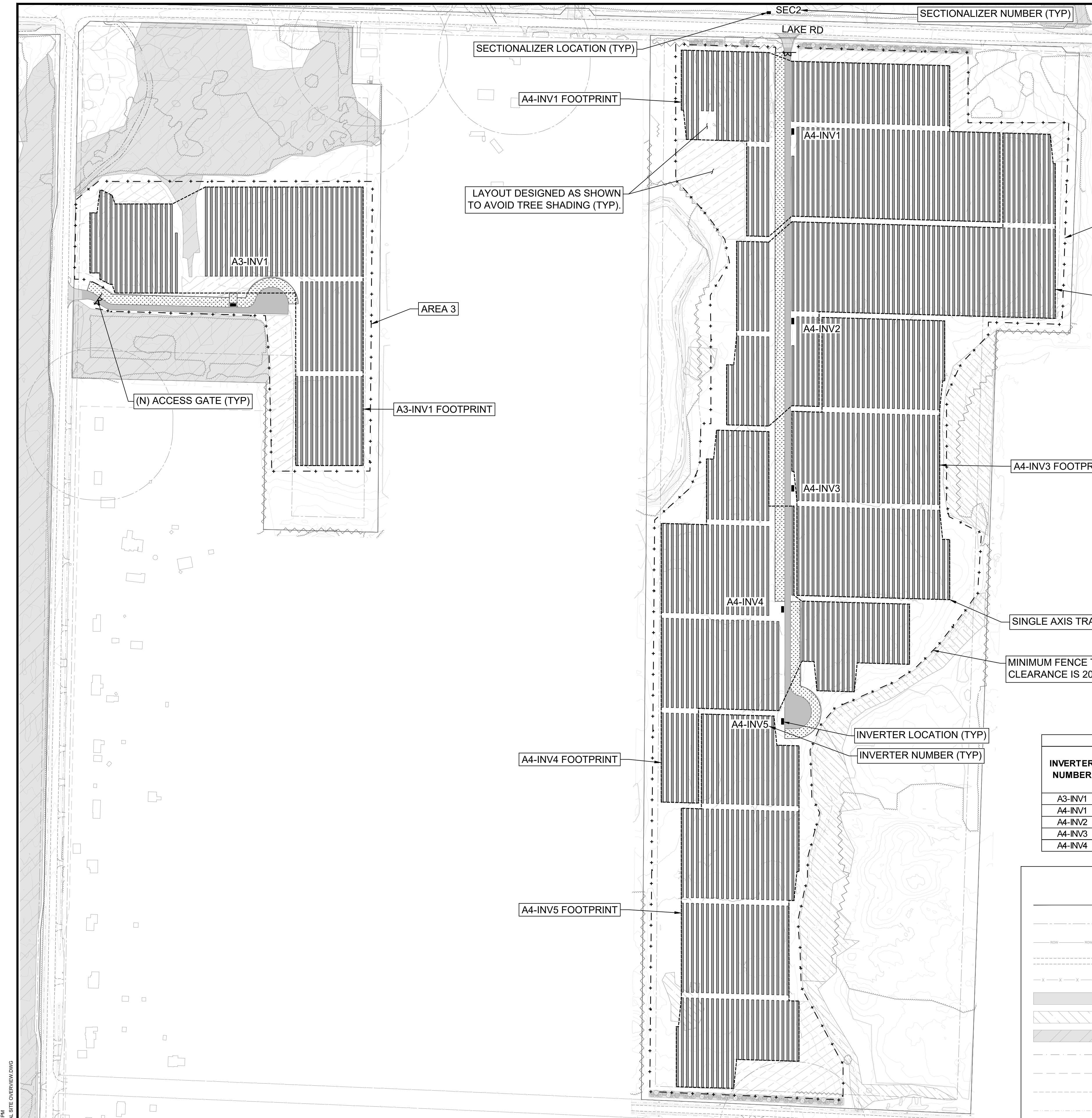
1 ENLARGED ELECTRICAL PLAN - AREAS 3 AND 4 SCALE: 1" = 200'
